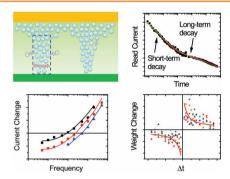
Internal dynamics of oxide memristors allow the device to implement different rate- and timing-dependent plasticity rules naturally in a biorealistic fashion with simple, nonoverlapping spikes.
