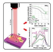
High-performance transition metal dichalcogenides (TMD) photodetectors are enhanced by self-assembled monolayer (SAM) doping. The photoresponsivity of WSe<sub>2</sub> and MoS<sub>2</sub> photodetectors is improved by a factor of ≈28.2 (with OTS p-doping) and ≈26.4 (with APTES n-doping), respectively. These improvements are attributed to the enhancement of TMD optical properties by SAM doping and this is also investigated in detail through photoluminescence analysis.
