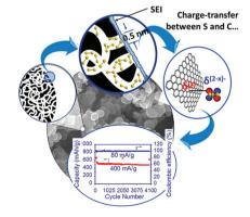
A new sulfur chemistry is created with the sequestration of short-chain sulfur species into subnanometer cavities and the charge delocalization between them and the carbonaceous host. Highly reversible capacities achieved at almost 100% Coulombic efficiency over 4020 cycles are demonstrated. This new charge/ discharge mechanism opens up new possibilities for designing nanostructured cathode materials for rechargeable Li/S battery chemistry.
