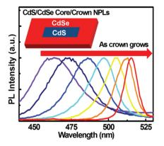
Continuously tunable photoluminescence in a model platform of inverted core/ crown nanoplatelets is demonstrated with a tunability range of 90 nm. The unique continuous tunable emission is achieved by controlling the lateral width of the CdSe crown around the seed CdS nanoplatelet template because of the finely tuned lateral quantum confinement in the crown region additional to the pure vertical confinement.
